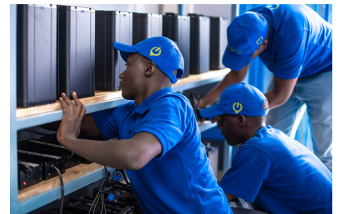
Employees attach battery packs to charging points. Photo: Spiro
