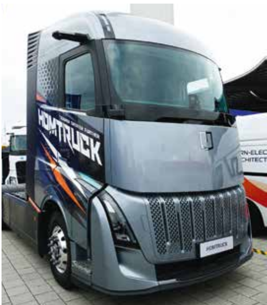
The Farizon Homtruck: a modern design with 600 kWh, a 500 km range, and an electric axle. It would actually be a strong contender for the European market if it were also available as a 4x2 tractor.
