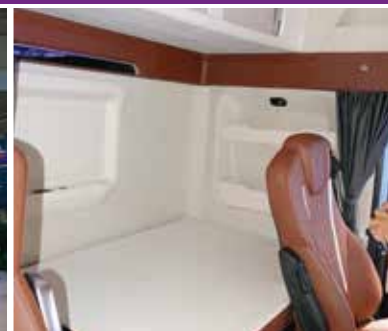
The new Foton Cavan Beacon offers plenty of living space: Its excellent aerodynamics allow for a deep cabin with a 90-cm bed and spacious storage cabinets on the rear wall—even for Europe.
