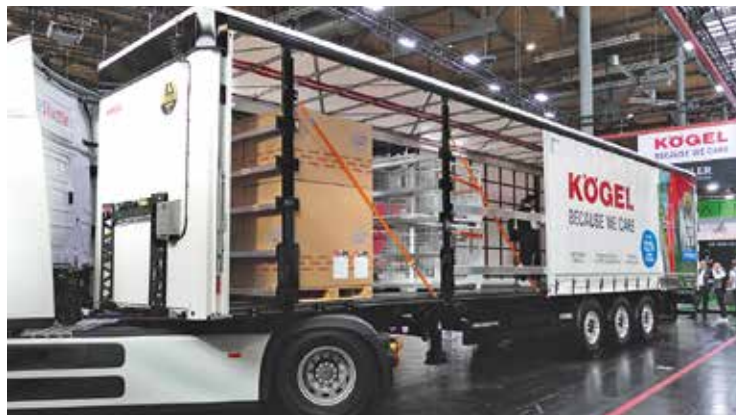
The e-optimized Curtainsider Light Plus reduces the load on the drive axle of heavy electric tractors by a good metric ton thanks to a three-axle unit mounted 30 cm further forward. The forward-mounted front wall also reduces the load on the drive axle and allows for up to 20 percent—or four metric tons—more payload with appropriate load distribution.
