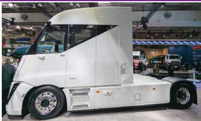
Foton: The Cavan Beacon was unveiled at the IAA. Entry behind the front axle, electric axle from ZF. With a wheelbase of 4,800 mm, will there still be room for a standard 13.6-meter trailer?
